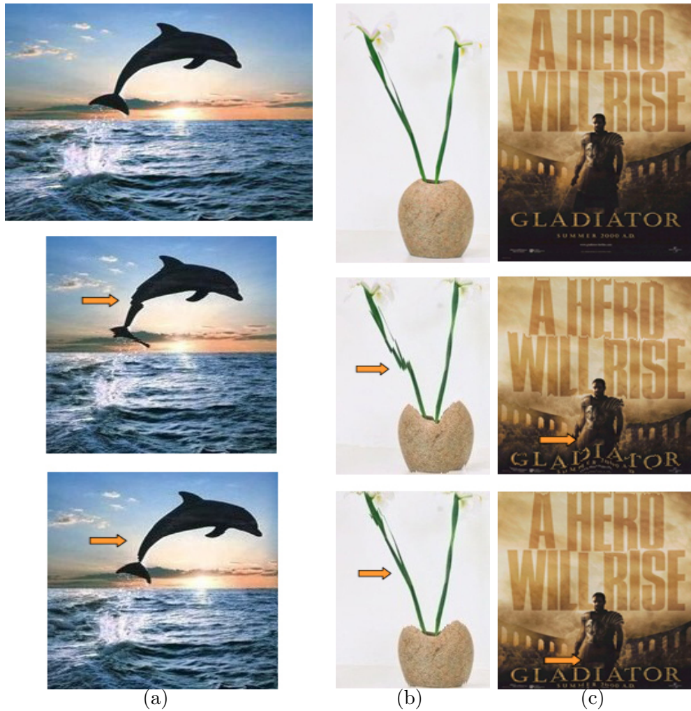
Figure 4.24: Image resizing using graph search method. The first row is the original image. The second row is the graph search result without the shape prior penalty. The third row is the result with the convex shape prior penalties. Typical improvements are pointed out by arrows.
